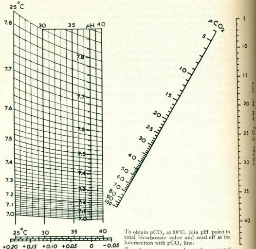
CORRECTION FACTOR to be added to pH values determined at 38°C. to give pH at t°C.
